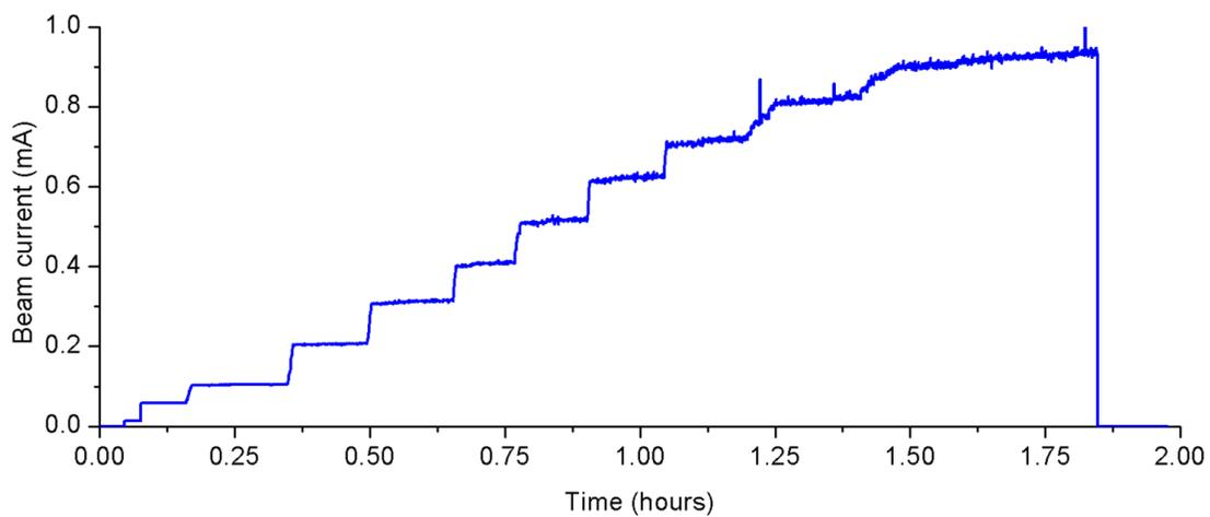
*Fig. 4. Typical signal of current in time while raising the laser power to obtain 1 mA.*
