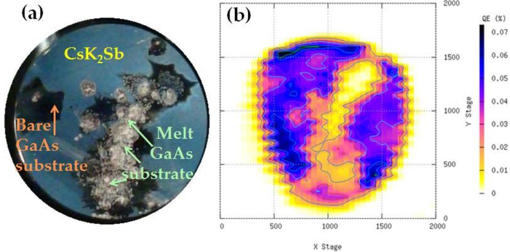
Fig. 8. (a) Damage at the electrostatic center of the PC caused by a series of arcing events. With anode biased from 0 to +1500 V. (b) QE map of the PC shown in (a).
