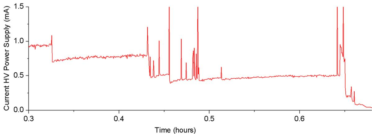
*Fig. 7. (a) Current at the HV-PS during a series of arcing events. Each spike represents an arcing event. Even after several AE the photocathode still provides beam current.*
