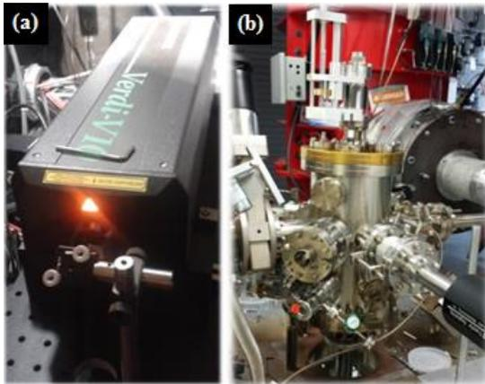
Fig. 1. (a) 10 W Coherent Verdi laser, (b) photocathode preparation chamber and (in red) the High Voltage Power Supply for the electron gun.
