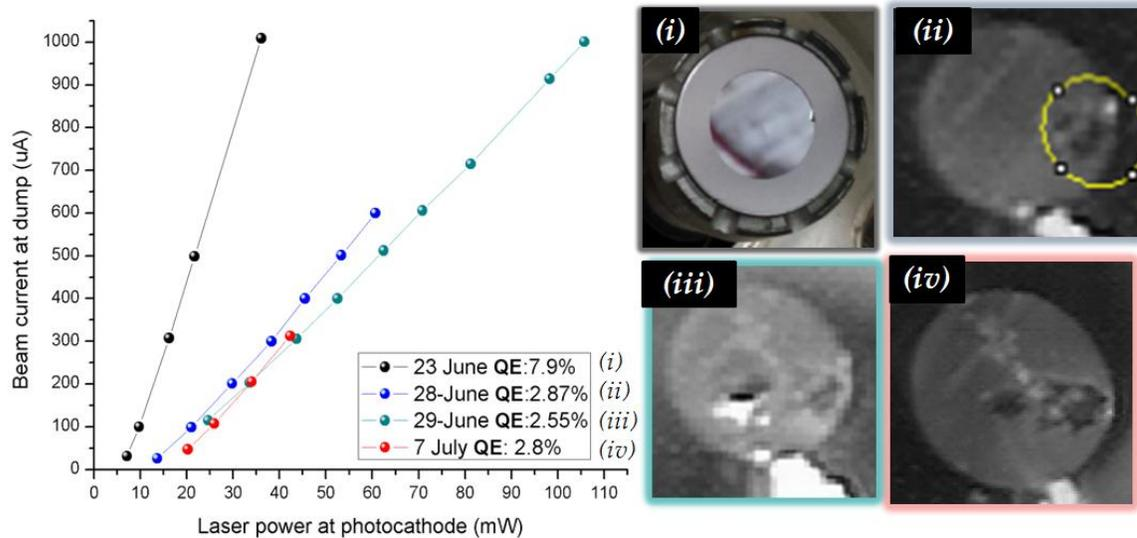
Fig. 9. QE curves for different EB runs (left). Laser spot was located at a non-damaged area to obtain the curves. Each QE curve is related to a PC image where the different damages are visible (right). QE barely changes after arcing damage at non-damaged spots.
