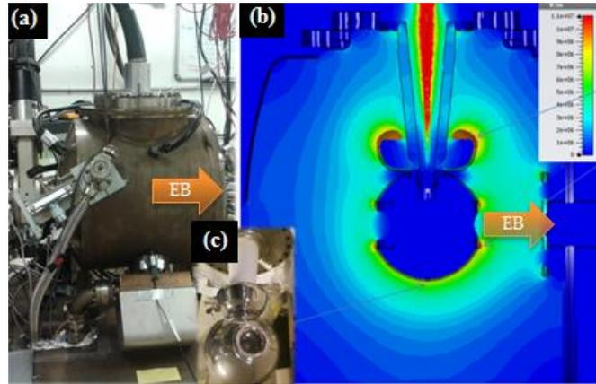
Fig. 2. (a) Inverted-geometry DC electron gun picture, the arrow shows the EB direction. (b) Interior of the electron gun, the color represents the voltage, the electrode is the sphere in the center and the anode is at the end of the arrow. (c) Electrode picture.
