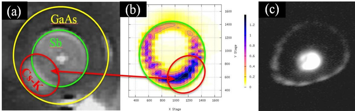
*Fig. 10. (a) Picture of a masked photocathode fabricated to reduce EB halo by limiting the active area. The bright point in the center is the laser beam. (b) QE scan of the masked photocathode. (c) Picture of the EB generated by locating the laser spot at the center of the masked PC.*
