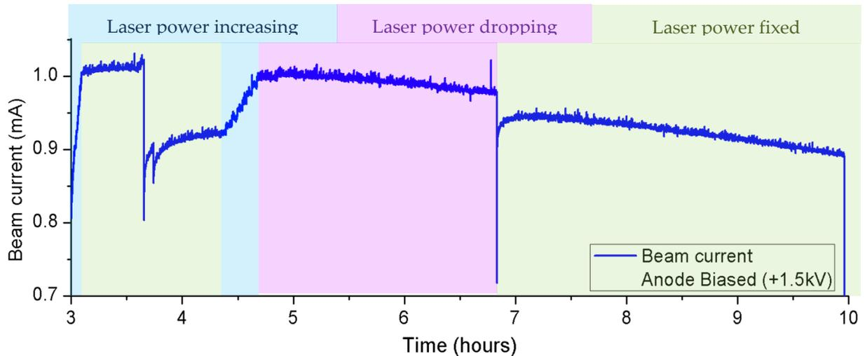
Fig. 6. EB run at 1 mA for ~ 6 hours. Each current drop was caused by an arcing event. Background colors indicate the laser power status: blue– laser power (LP) increase; green – LP fixed; purple– LP drop.
