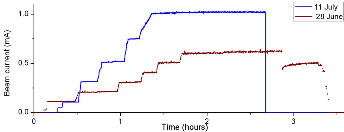
Fig. 5. EB run at 0.6 mA and 1 mA for more than 1 hr. The runs were stopped due to HV-Power Supply (PS) trips. There is no observable QE decay with time. The QE decay for the 0.6 mA run was caused by an arcing event.
