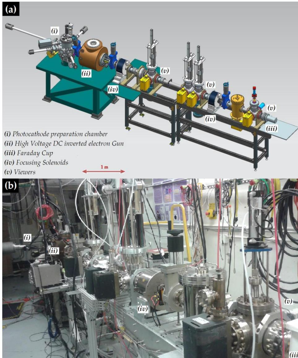
*Fig. 3. (a) Beamline schematic. (b) Gun Test Stand (GTS) beamline picture. Our PC is fabricated at the preparation chamber (i), and then it is introduced to the HV-DC electron Gun (ii). The EB is produced by shining green laser light on it. Then it is focused (iv) and steered with magnets to the Faraday cup (iii) at the dump of the beamline. The Faraday cup collects beam current. The beam shape can be observed through the viewers (v).*
