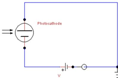
Figure 2: Bias system used, anode biased at ~1360 V.
