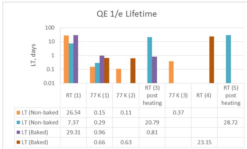
Figure 4: Lifetime of photocathodes at different temperatures in two vacuum conditions.
