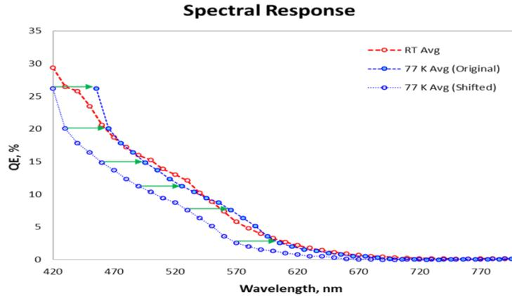
Figure 6: Wavelength shift equivalent to 35.6 nm when cooling the photocathode to 77K.
