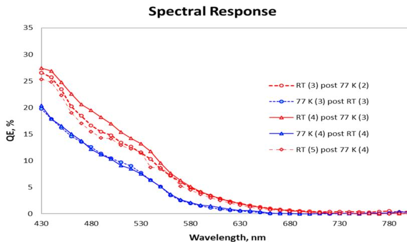
Figure 5: Spectral Response of QE at different temperatures.
