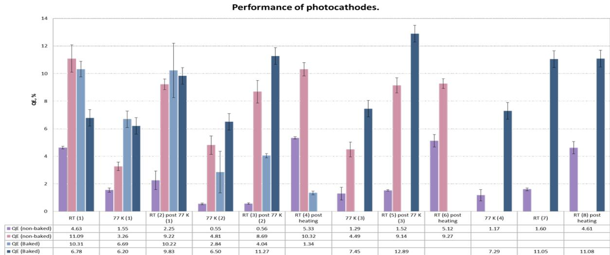
**Figure 3: Photocathodes QE performance at different temperatures in two different vacuum systems.**
